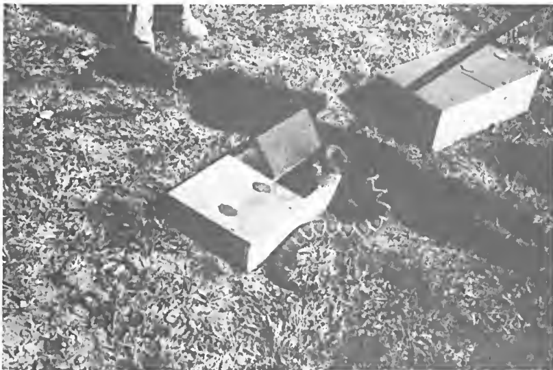
Fig. 5 — Photo Inst. Butantan — Box with 2 partitions for the transport of ophidians, standard model of the I.B.
